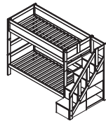
BUNK BED WITH STEPLADDER H 177 x W 257 x D 102/132 Ground clearance below the bed 25 CM Space between the beds 104 CM
